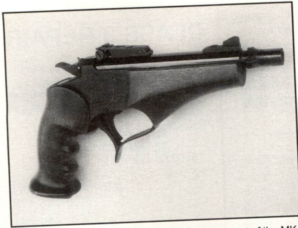
One of the test guns used during the development of the MK-26 suppressor was a Thompson Contender single-shot pistol fitted with an S.C.R.C. three-lug barrel.
