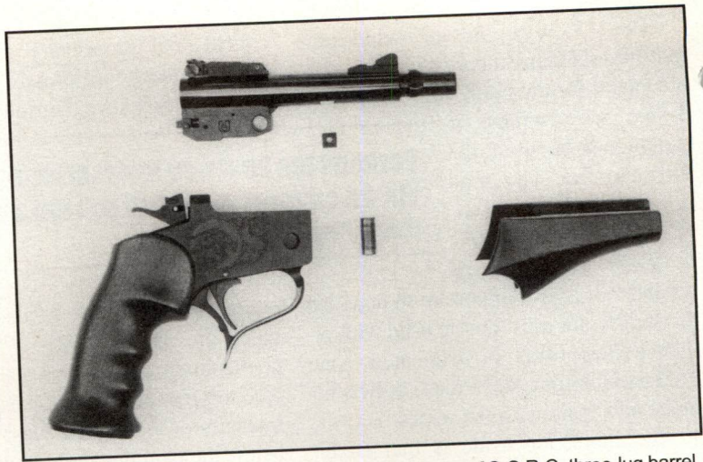
Field stripped Thompson Contender showing details of S.C.R.C. three-lug barrel.
